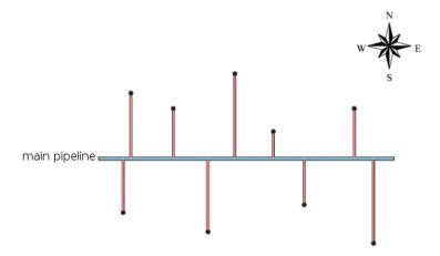
The main pipeline is represented by the horizontal blue line. The wells correspond to the dots and the auxiliary pipelines are the red segments linking the wells to the main pipeline. We wish to minimize the sum of the length of the red segments.
